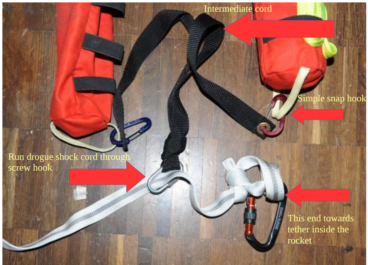
Picture 8: Main chutes assembly
