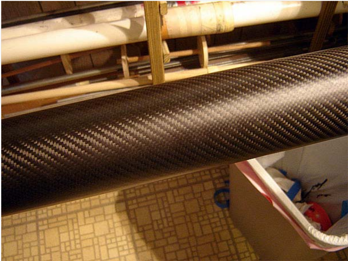
Here's the tube after wiping on the first coat of epoxy. You could almost stop here, but there is still room to improve the finish.
