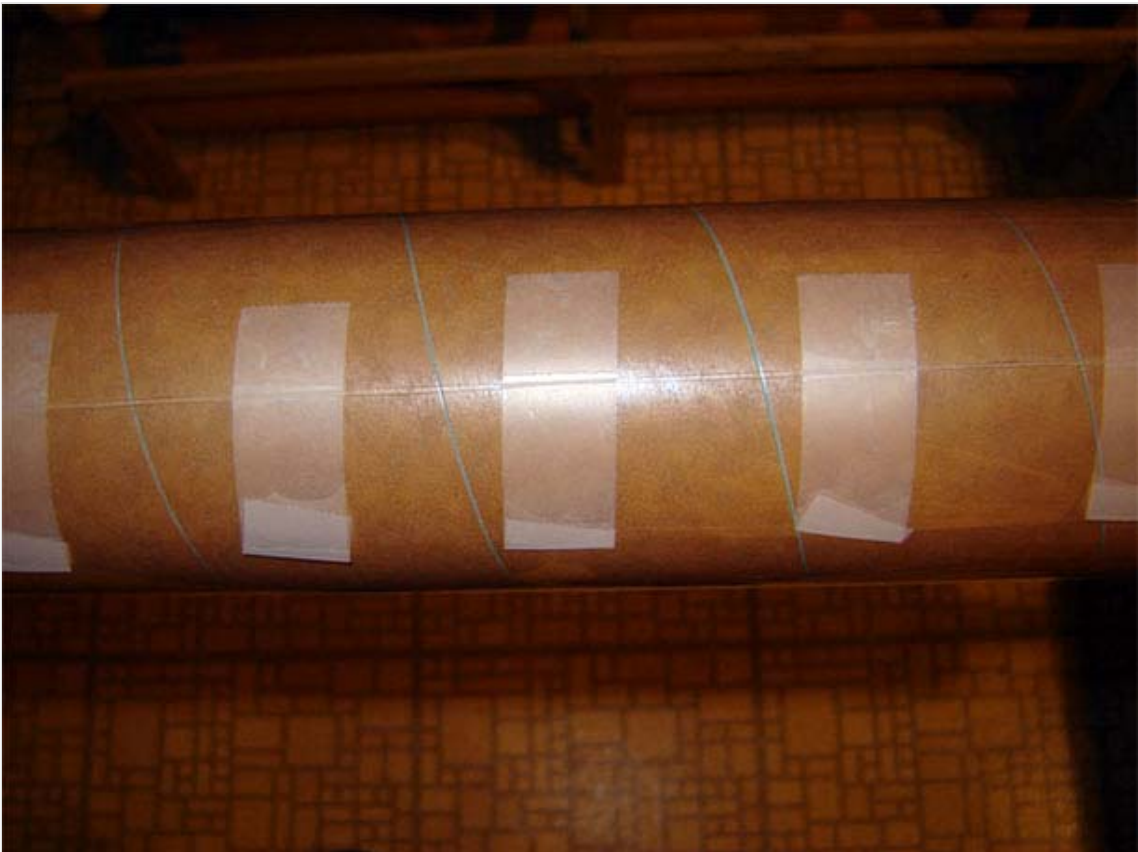
Here, the mylar has been wrapped around the mandrel. Note the 1mm gap. The mylar is wrapped as tightly as possible and secured with pieces of tape. I start in the middle and work toward the ends. Note the fold at the
