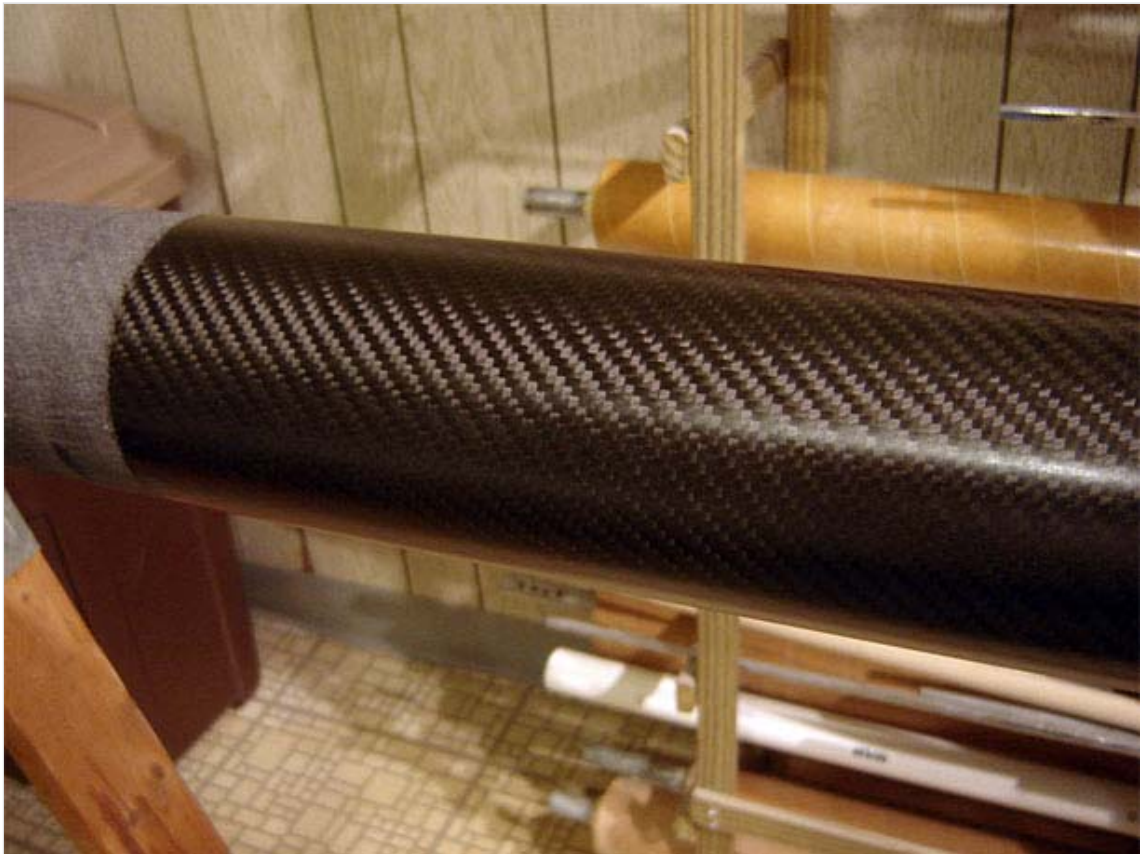
This is after the second wipe coat of epoxy. No sanding between these two coats.
