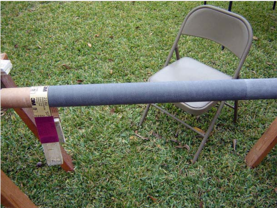
Here's the tube after 220 grit – not too many flaws! My shoeshine sander is on the left. I find this setup much easier
