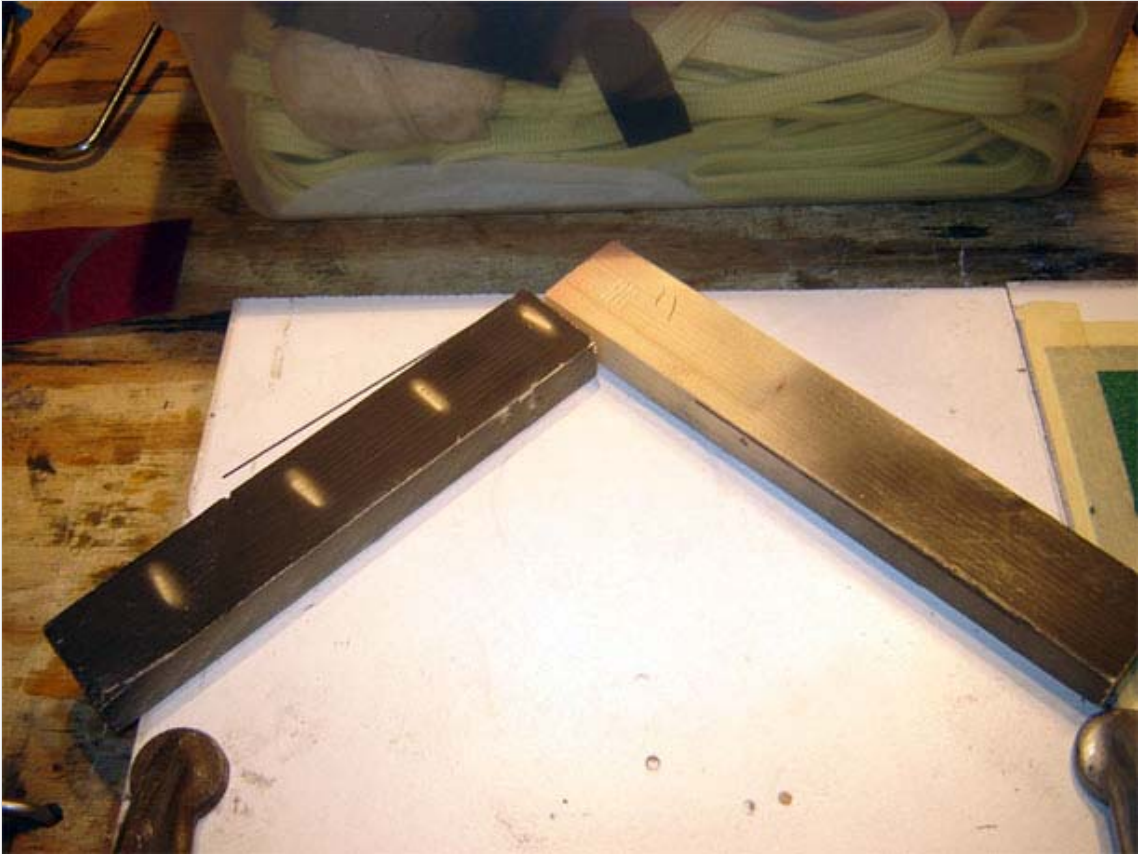
The flat board with the "V" shaped pieces is clamped to the workbench.
