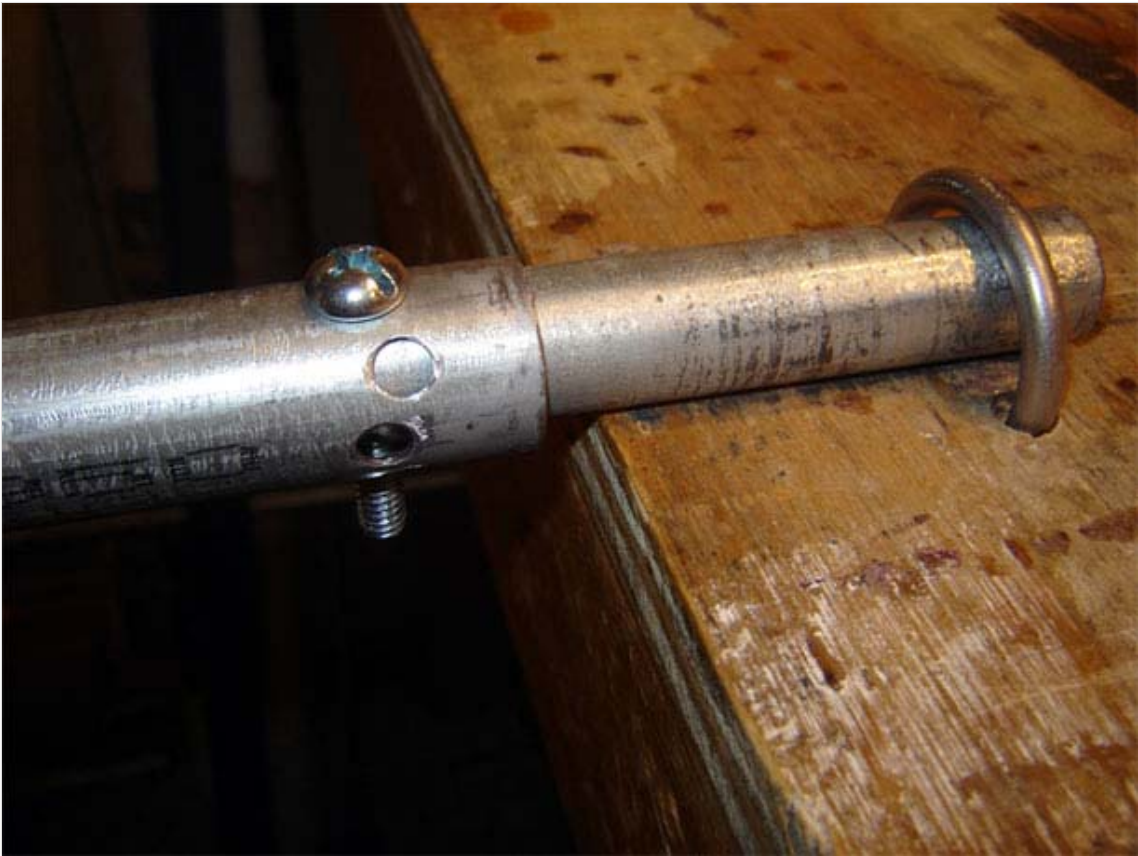
Here, the two tubes are "pinned" to hold everything solidly in place.
