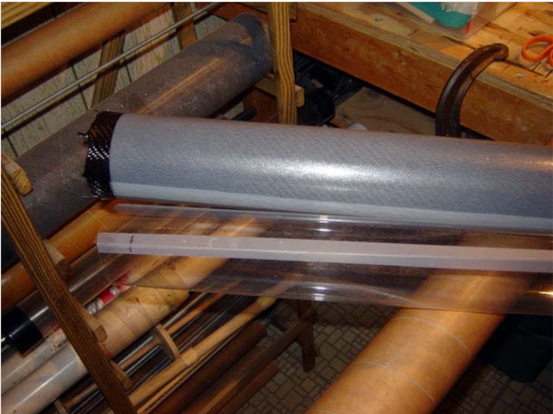
The mylar comes out next. By curing at only 90F, the mylar comes out easily.
