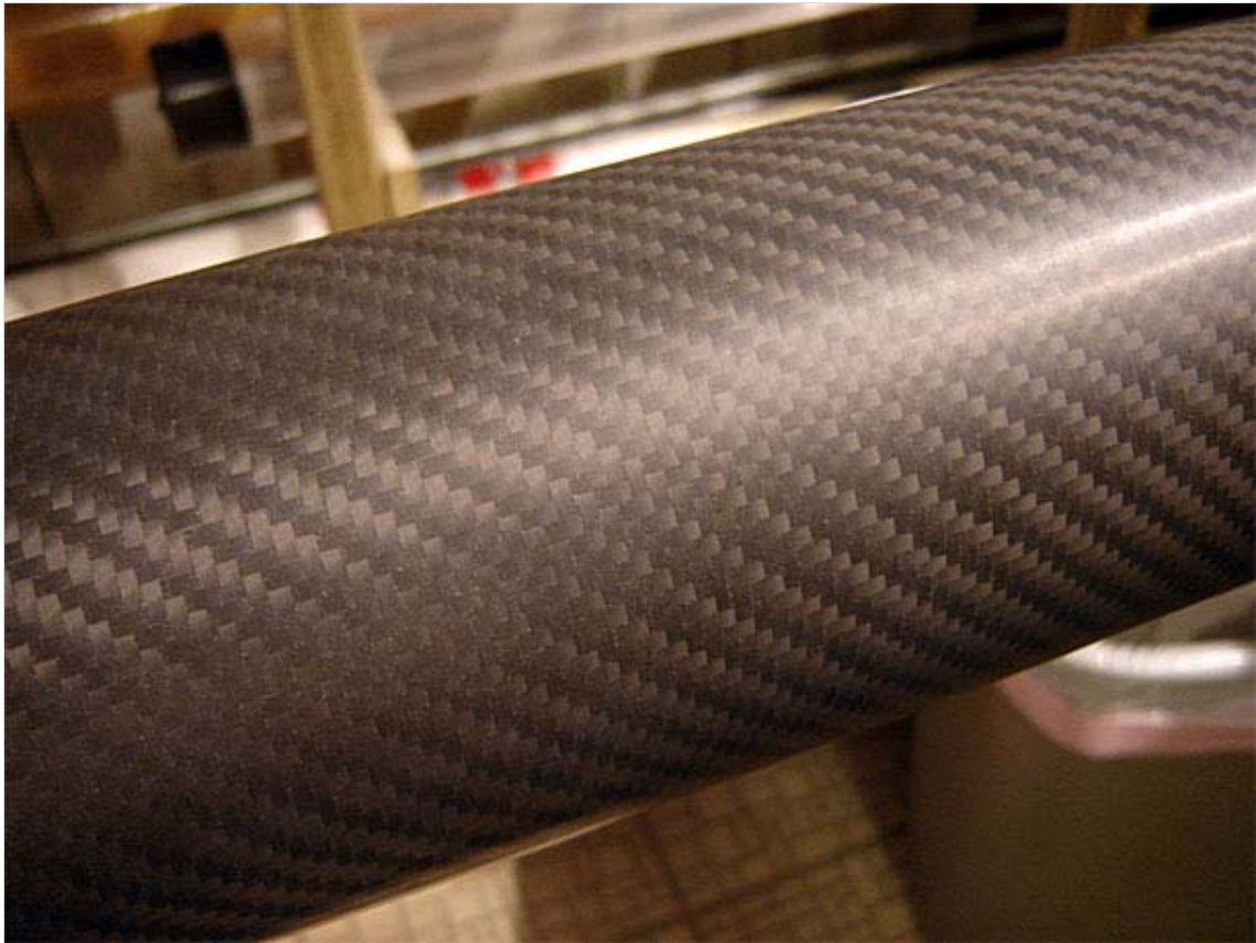
This picture was taken after one pass with 600-grit wet sandpaper. Note how the scratches have been filled by the epoxy wipes!
