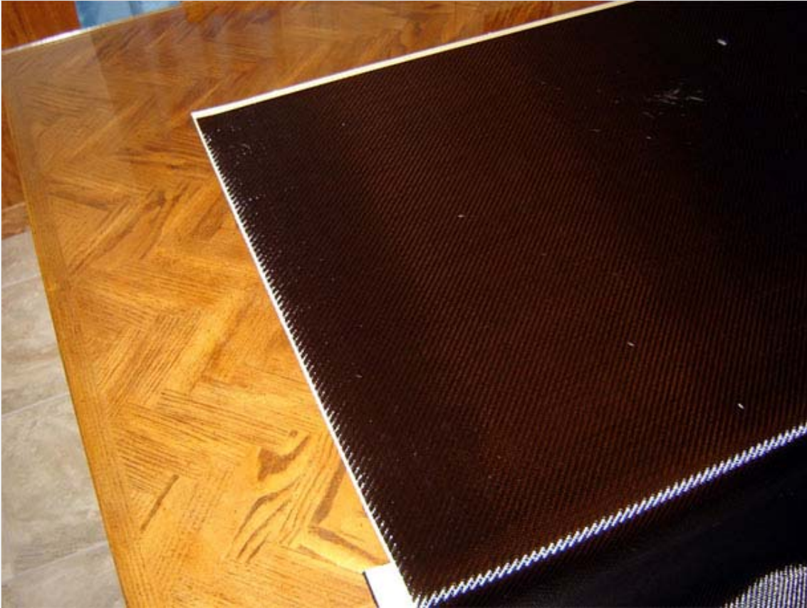
I use masking tape around the edges of the carbon to keep it from fraying. The widths are 1/8" at the point where the carbon is first applied to the tube, 1/4" along the sides of the carbon, and 1" along the last seam (this tape will be cut off later).
