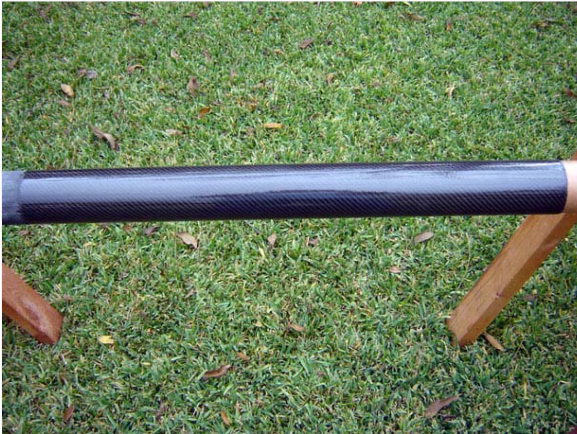
This is what the tube looks like after 6 coats of epoxy. Now, it's time to sand down the tube.
