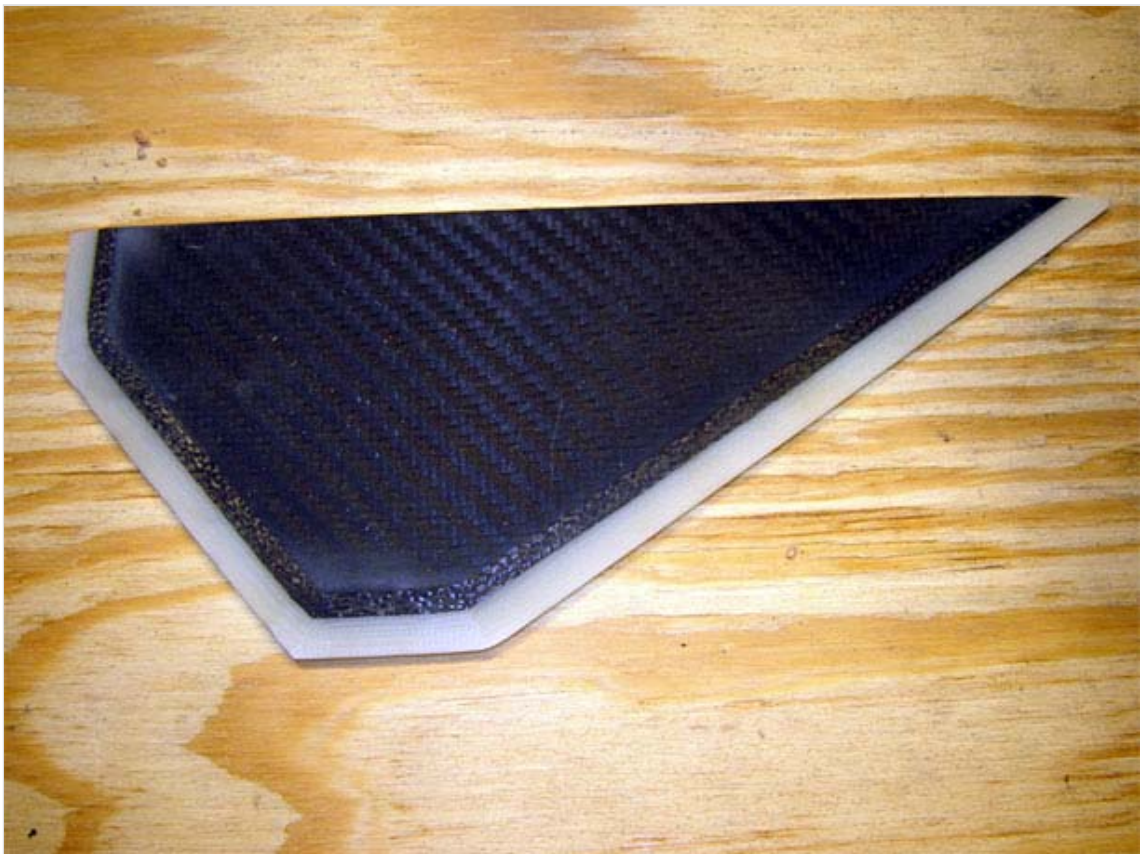
Here is the fin after sanding the first bevel around the perimeter.
