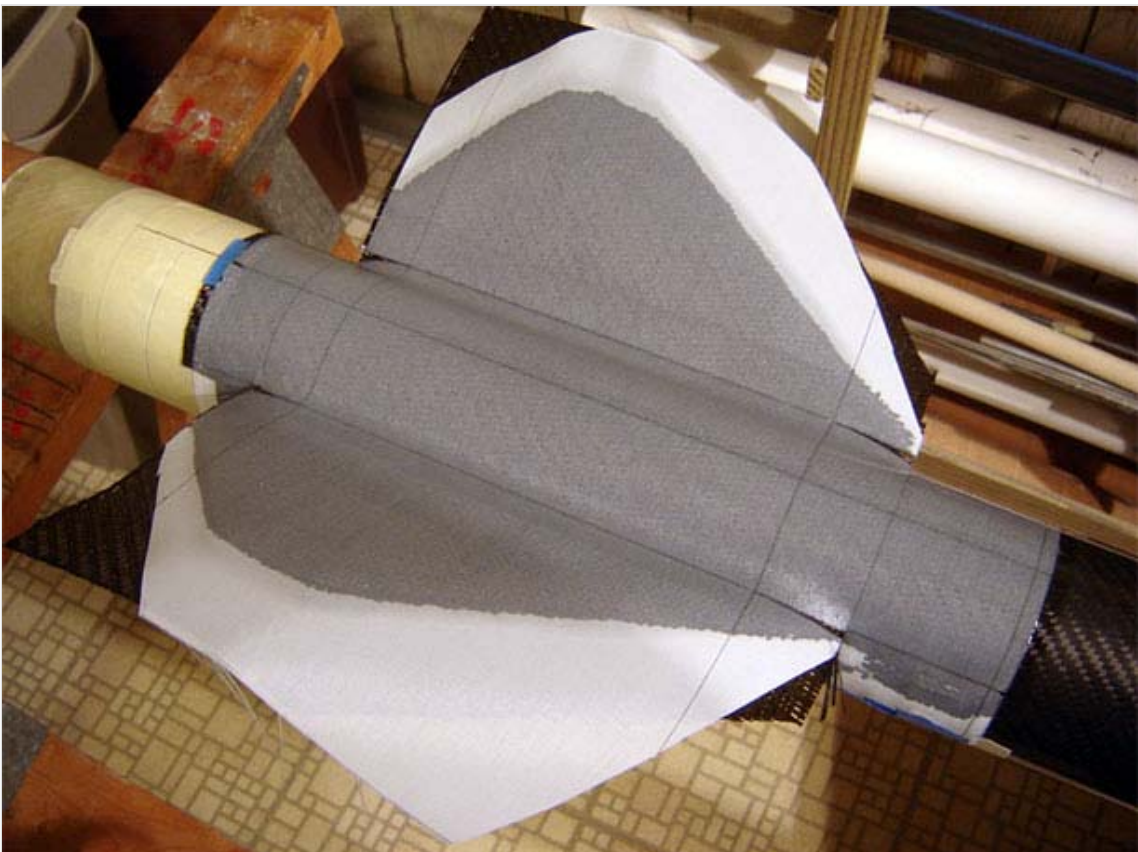
Here is the peel ply fully wetted out. As with the airframe itself, the idea is to remove the bubbles below the peel ply. This goes into the oven for an initial cure at no more than 90F.
