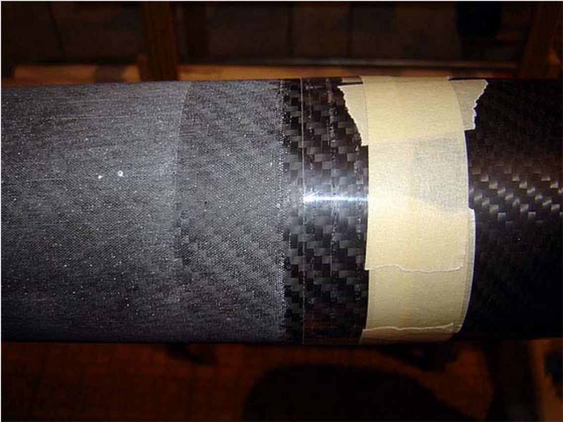
I use a piece of plastic as a sanding guide. The objective is to sand a channel to recess the top of the tip-to-tip carbon into the tube. Here, I've applied the plastic guide around the tube.
