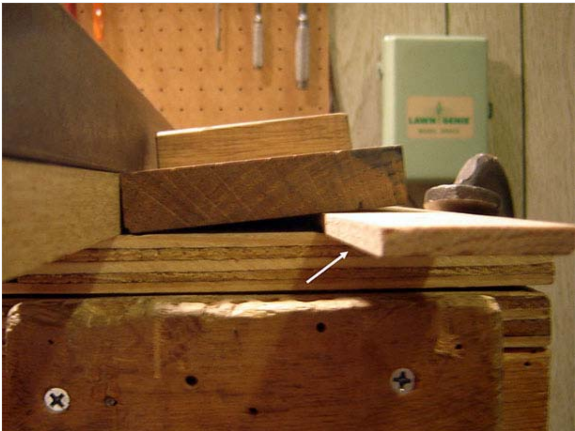
Next, one of the block is removed to cut a second bevel with \frac{1}{2} of the bevel angle (white arrow).
