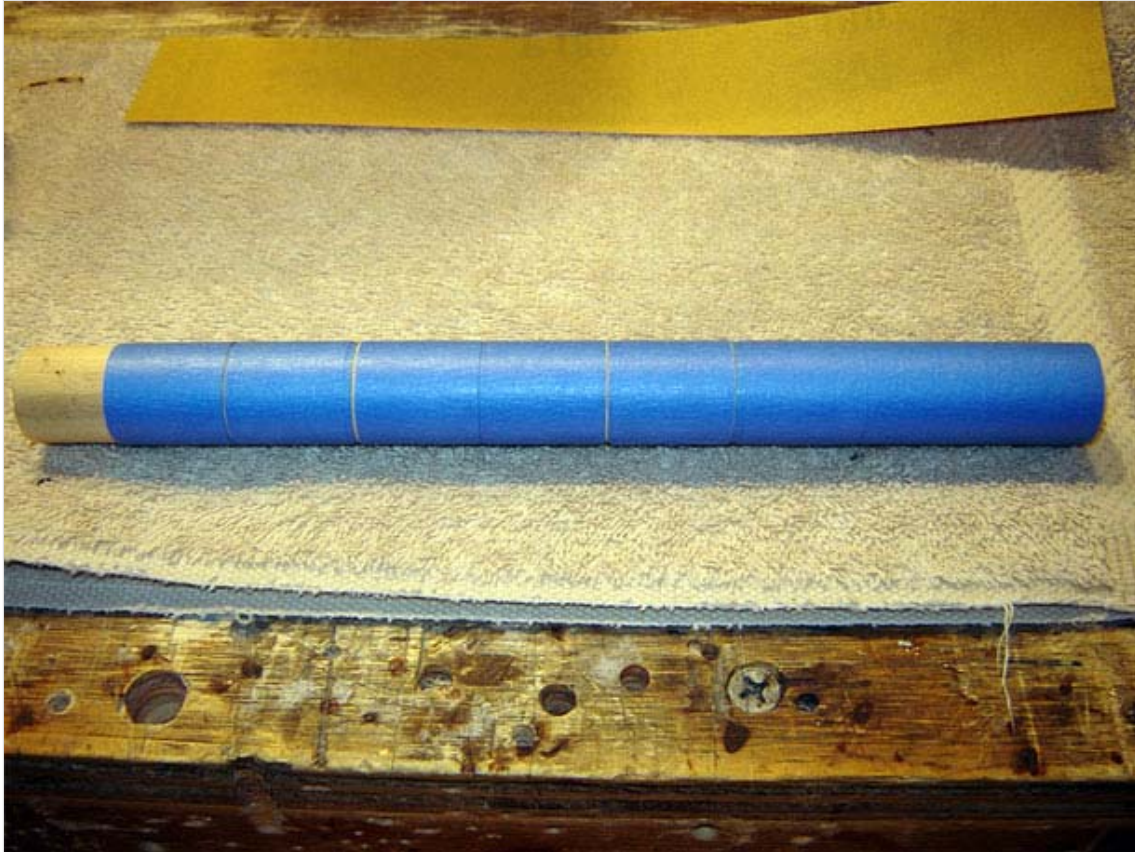
The original fillet was formed with a 0.97" dowel. I will sand it with a 7/8" dowel that is built up to 0.93" with tape. The 0.93" size is slightly smaller than the original fillet, which helps me to stay out of the carbon tube.
