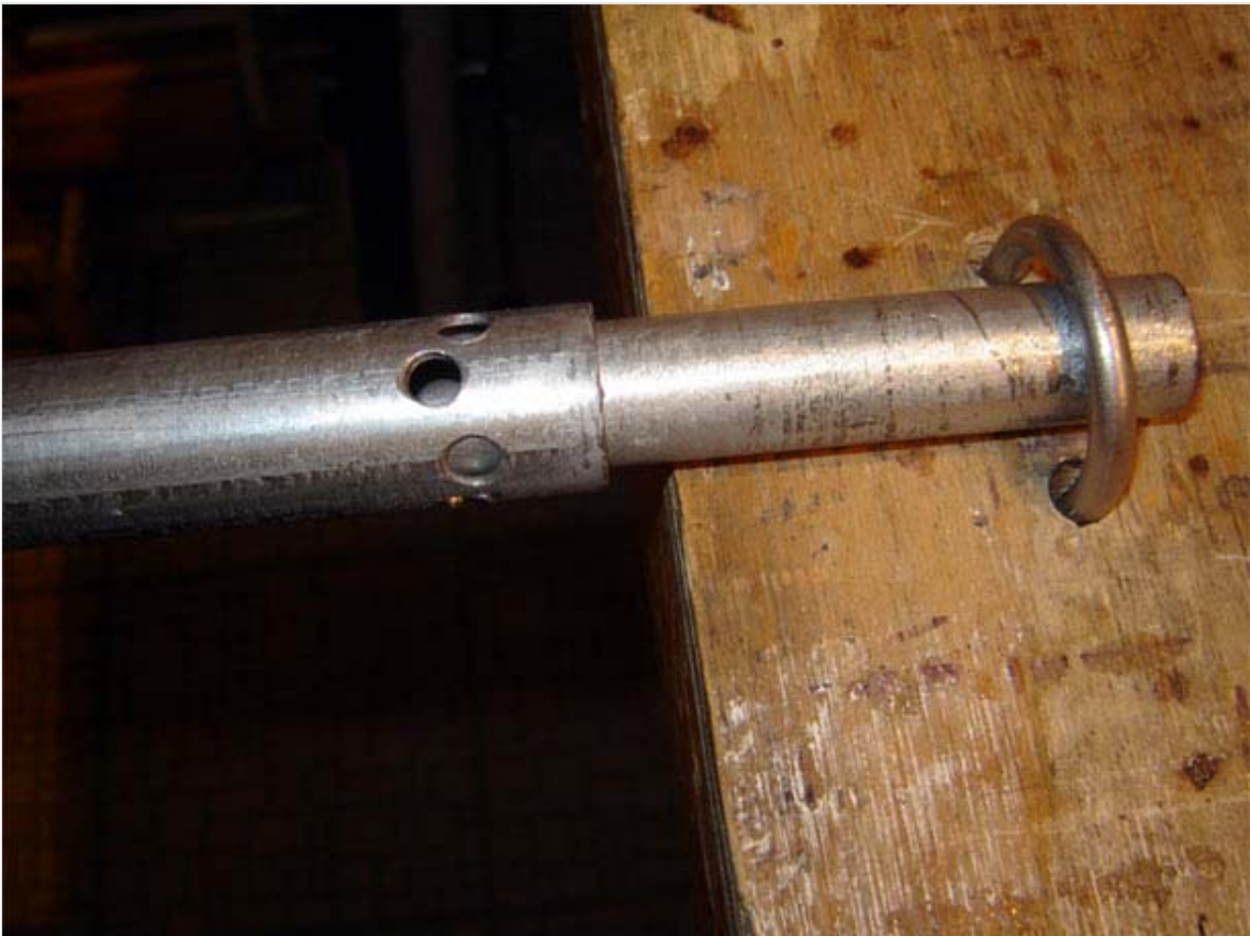
Here, the holes in the tubes are aligned. Note the U-bolt that holds the smaller axle to the work bench.
