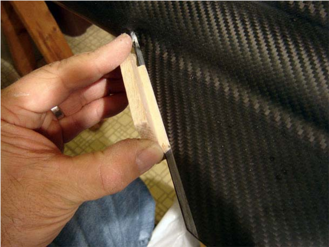
Here is a little right-angle jig that I made to sand the edge of the fin to a consistent depth.
