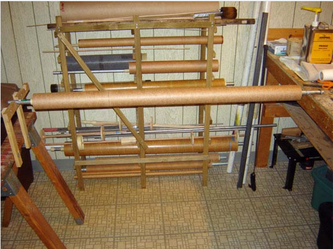
The whole tube is then filled with foam, and another ring is installed on the opposite end of the mandrel. It's now ready to work with.
