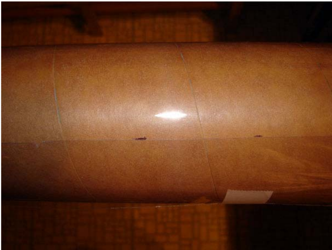
This is the 0.005" mylar wrapped around the mandrel. I have marked the overlap point, and I will cut the mylar so that it leaves about a 1 mm gap.
