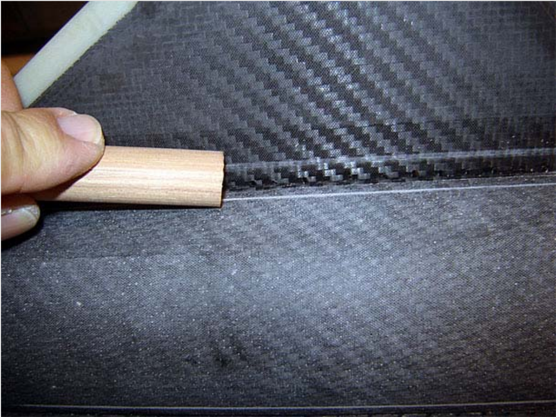
For making the fillets, I will use two dowels – a 5/8" dowel and a 1" dowel. Here, I'm using the 5/8" dowel to score lines for making the Cotronics fillets.
