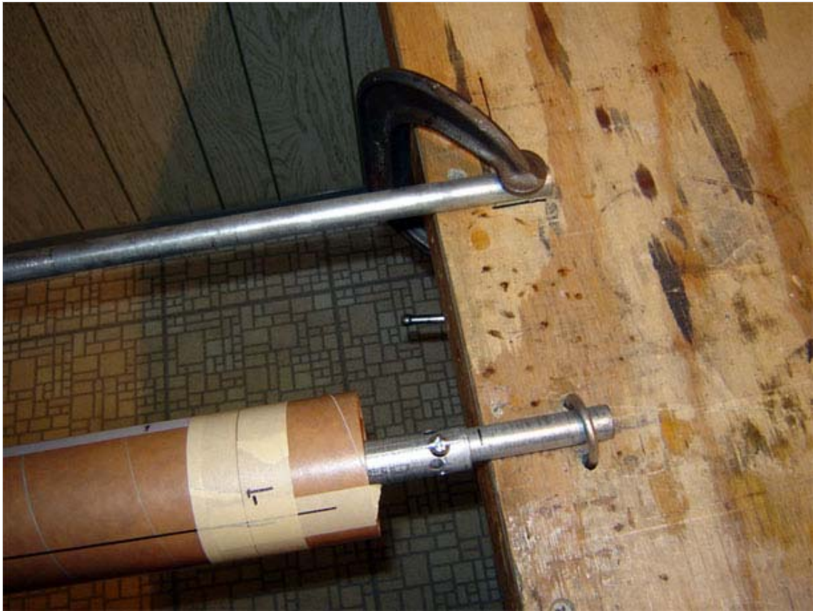
And the right side. The two rollers must be exactly parallel.
