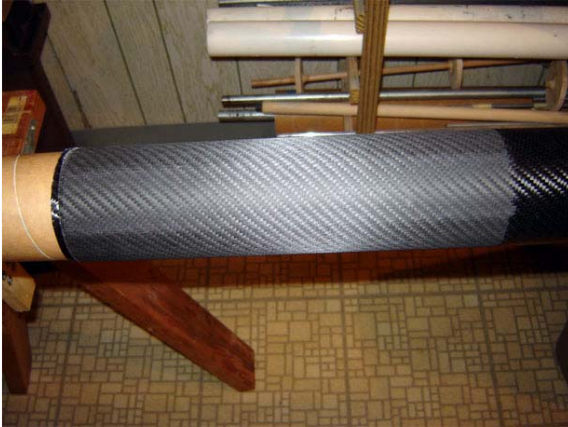
This is what the lower portion of the airframe looks like with the original peel ply finish and before any sanding.
