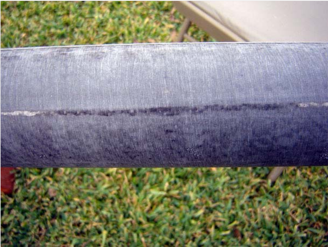
Here's the tube after the 180 grit paper. Much of the tube is smooth, but the seam area still shows some shine, and there are some small depressions below the seam area. But this is the time to go to the finer, 220 grit.
