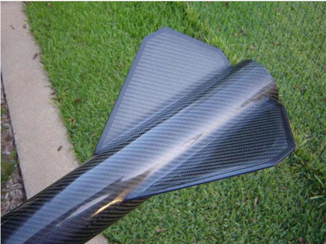
The original (with Cotronics epoxy applied to the fin edges).
