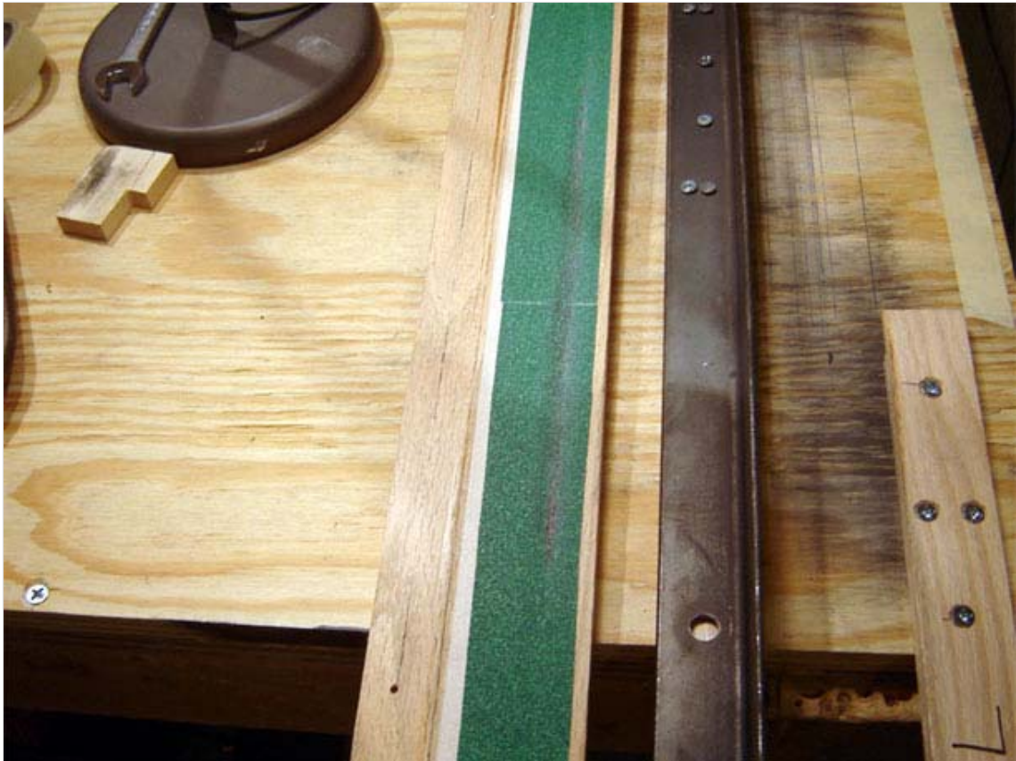
It has sandpaper attached with double-sided tape. The geometry of the jig must be carefully thought out.
