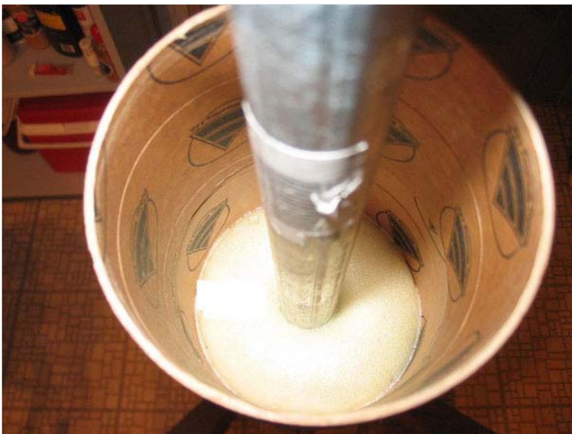
Filling the mandrel with foam to lock the "axle" in place.
