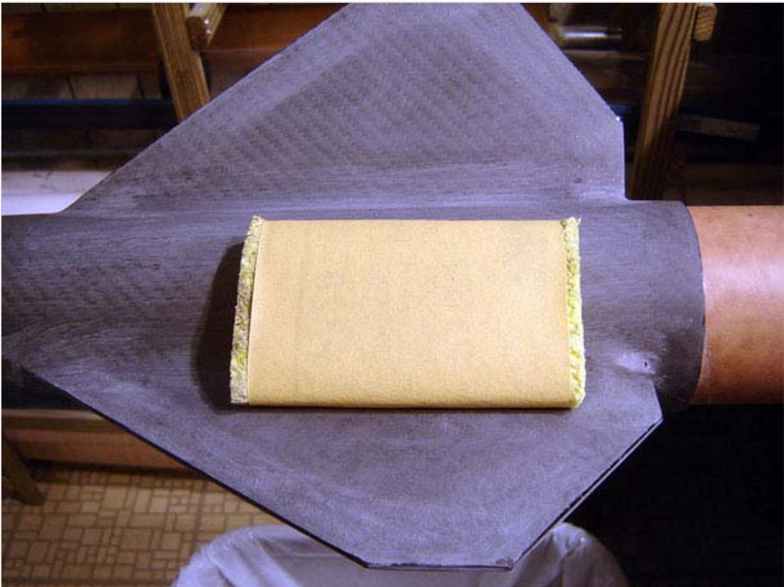
The entire fin can was first sanded with 180 grit paper using a sanding board for the fins, fin taper and body tube and dowels for the fillet and fillet transitions. In retrospect, I should have used 320 grit with the dowels, as some of
