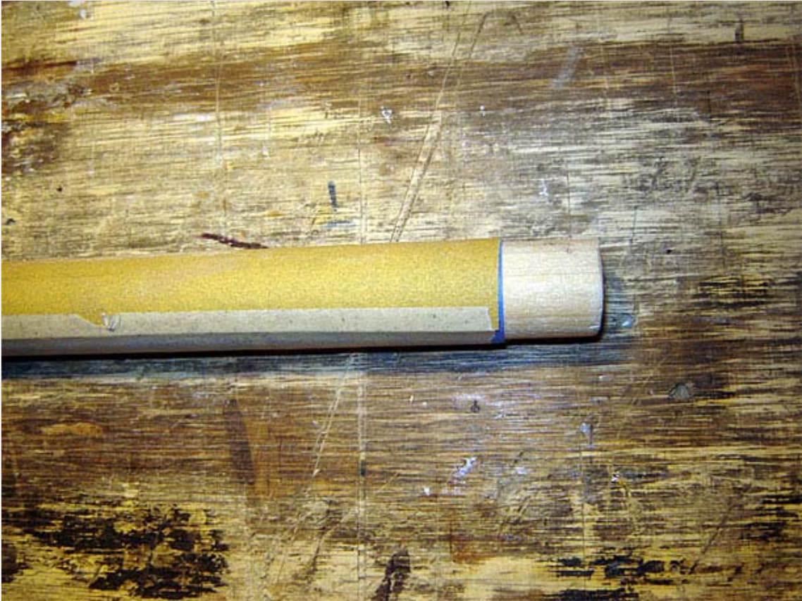
The sandpaper is taped on so that about 180 degrees of the dowel is covered. I used 180 grit for sanding the Aeropoxy Light filler.
