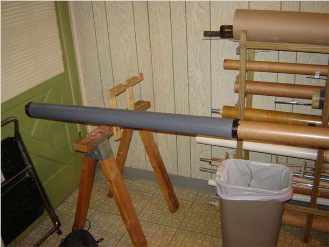
After curing for 24 hours, I trimmed back some of the carbon and then pulled the tube off the mandrel. It was not easy to remove!
