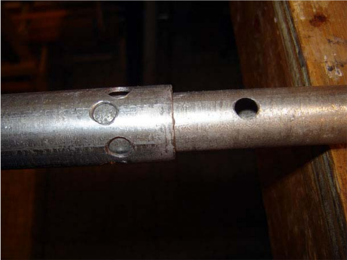
Note the 8 quarter-inch holes in the larger tube and the 2 quarter-inch holes in the smaller tubing.
