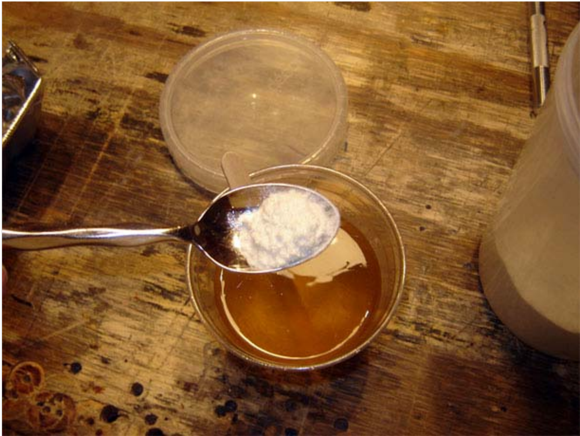
I add about this much milled glass to 100 grams of epoxy.
