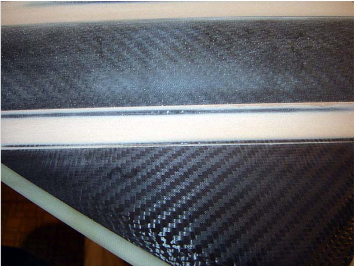
Here is the fillet after sanding with the slightly undersized dowel. All of the fillet surface has been "hit", and the
