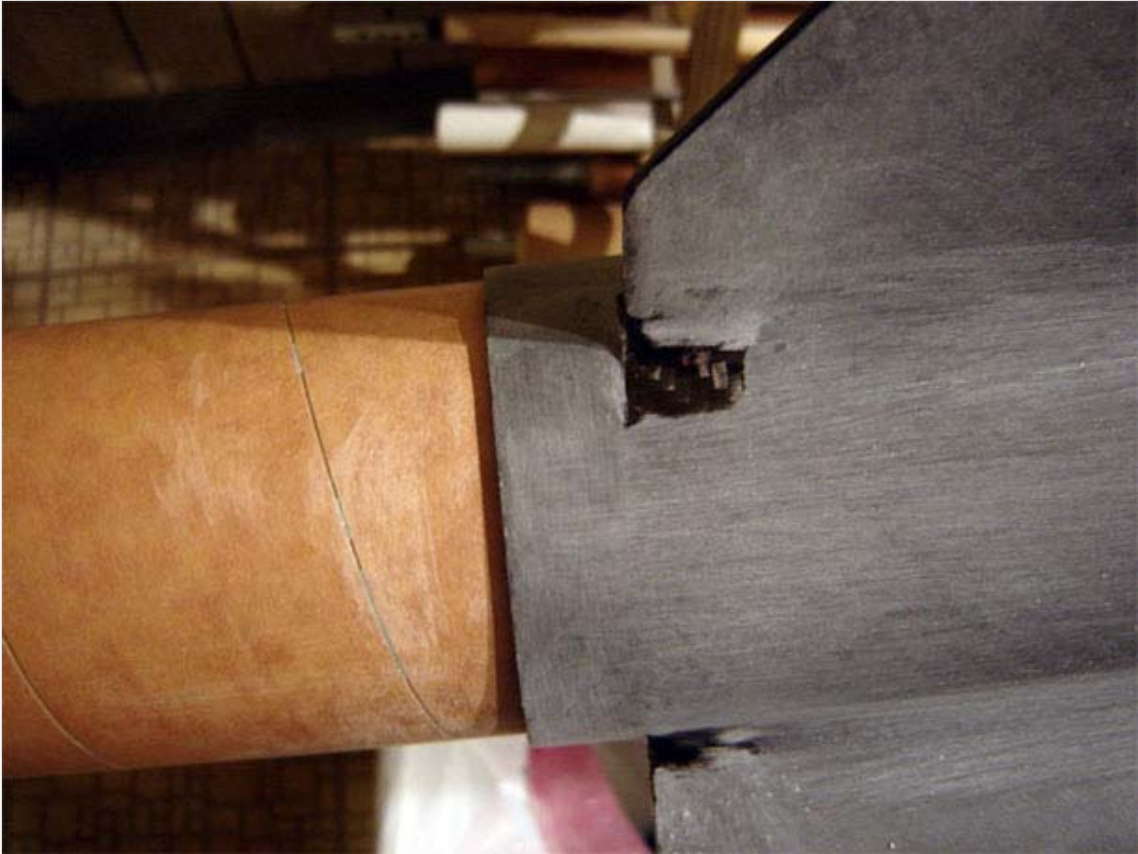
The same basic process is used to sand the aft end of the airframe below the fins.
