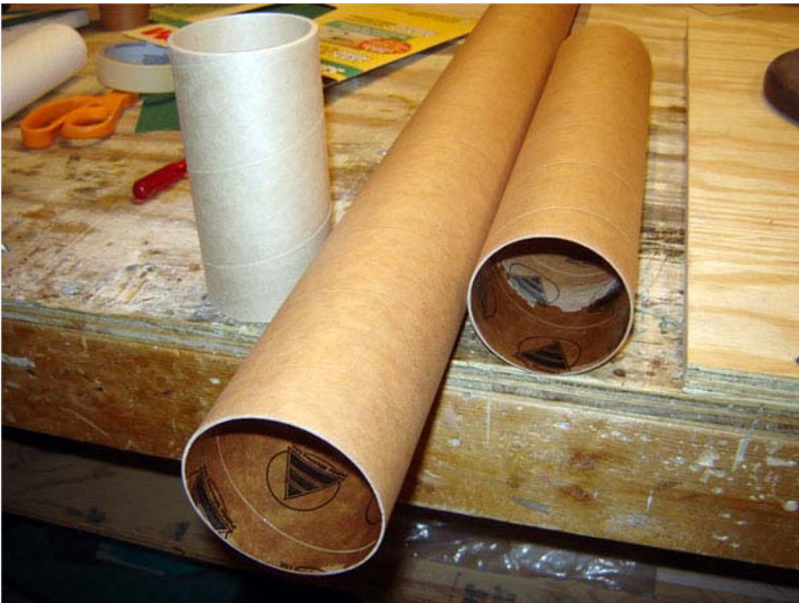
Here are the PML coupler tubes and the LOC "stiffy" tube that fits inside of the coupler tubes. The inside of the coupler tubes were sanded and epoxy has been applied.
