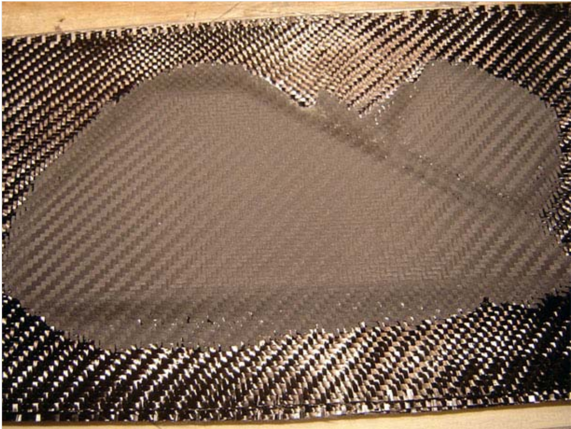
Peel ply removed.
