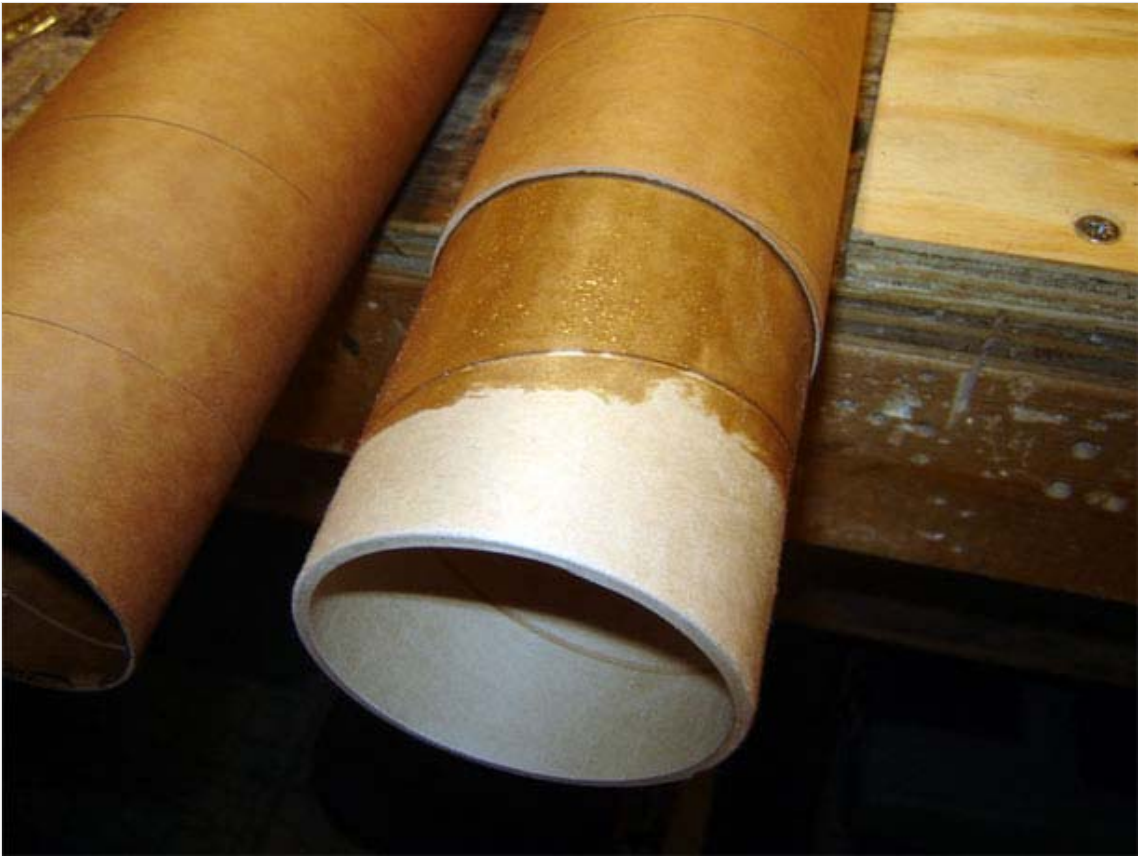
The stiffy tube installed with epoxy being applied.
